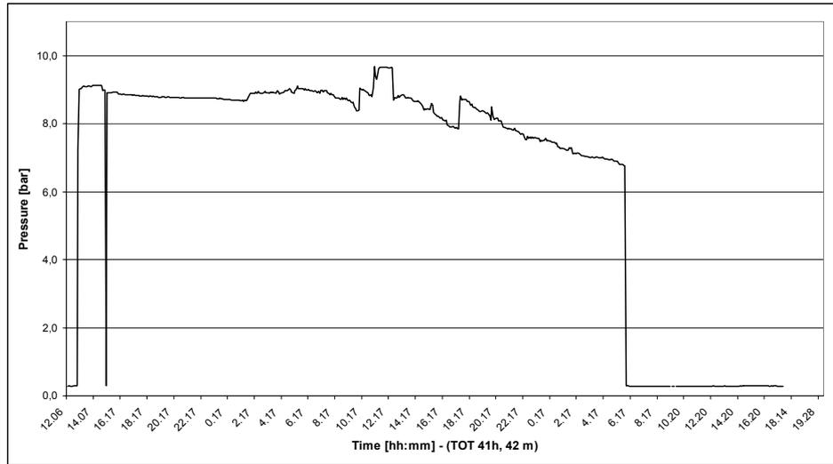
Fig.7 Pressure at pump outlet during the PO-LFO pump test
