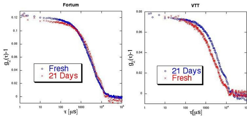
Fig. 2 Fresh emulsion (red) and 21 days aged (blue) emulsion obtained by micronization at 70°C of Fortum (left) and VTT (right) POs (30%) and Diesel Oil (70%). X axis:  $\tau$  [ $\mu\text{s}$ ] is the delay time; Y axis:  $g_2(\tau)-1$  is the autocorrelation function of the scattering intensity. In the Fortum case, the aged curve is almost identical to the fresh one
