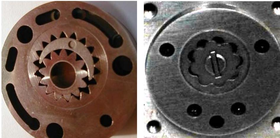
Fig. 4 Gears of the Suntec pump (left) and Delta pump (right).
