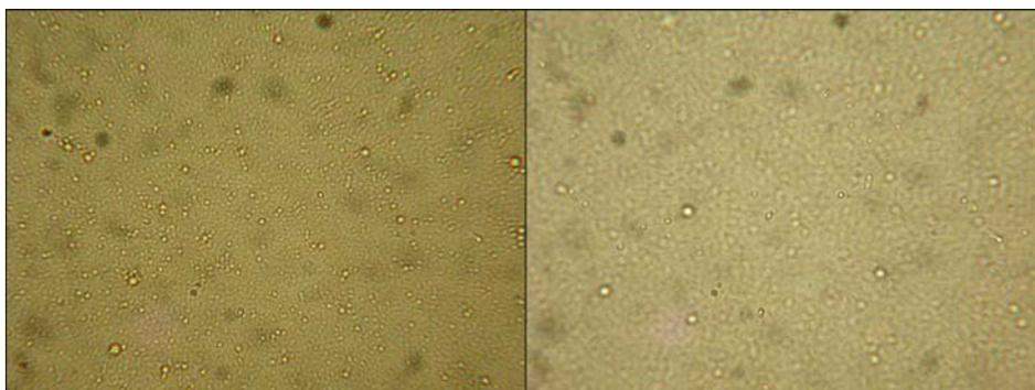
Fig. 1 Fresh emulsion (left) and 20 days aged (right) emulsion obtained by micronization of FORTUM PO (30% w/w) and LFO (70% w/w). Average diameter of the droplets is about 2  $\mu\text{m}$ .
