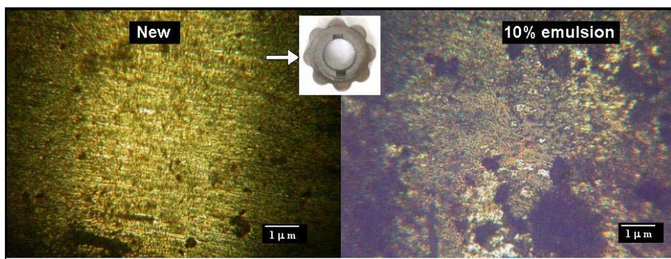
Fig. 9 Cog surface after pump test
