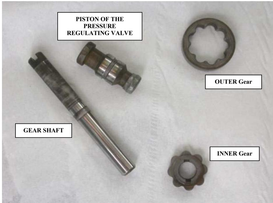
Fig. 8 Pump components under investigation
